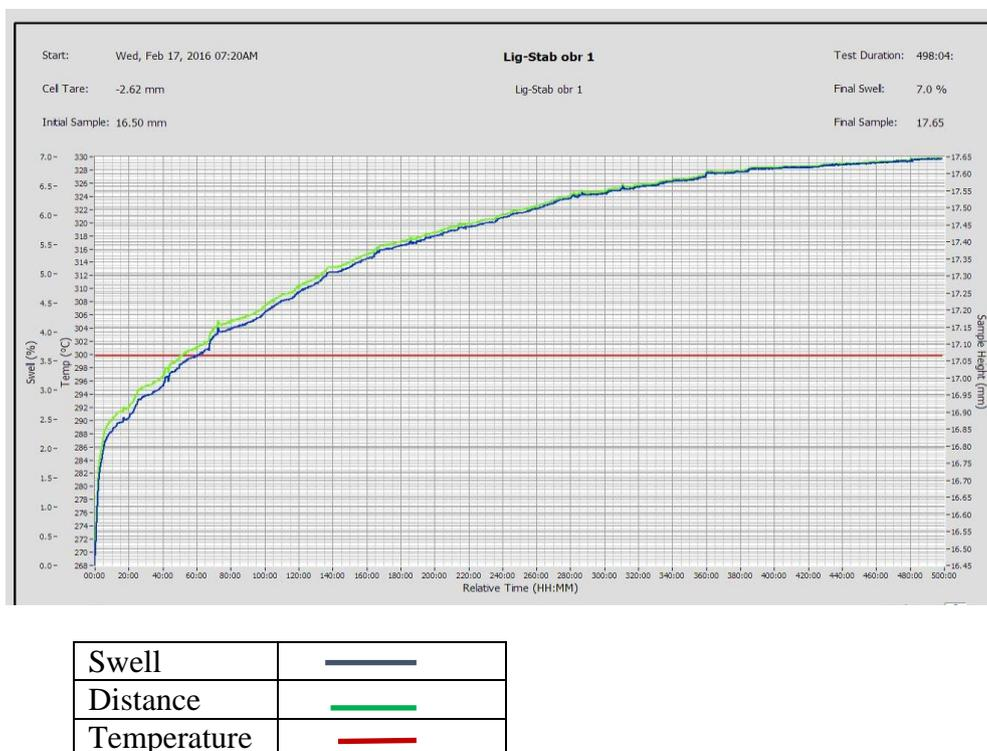
Fig. 1. Swelling curve of Kynov argilliferous deposits in biopolymer potassium chloride biopolymer drilling fluid containing the inhibitor of shale “LIG-STAB”
