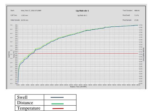
Fig. 1. Swelling curve of Kynov argilliferous deposits in biopolymer potassium chloride biopolymer drilling fluid containing the inhibitor of shale "LIG-STAB"
